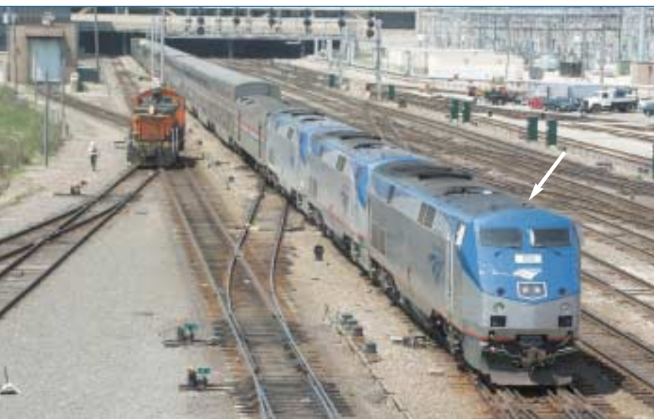
As Amtrak's California Zephyr leaves Chicago Union station, the DGPS aerial for the PTC pilot project is visible on the roof of the lead loco (arrowed), although this particular train will not traverse the Mazonia – Springfield route Photo: Ron Goodson/www.railnut.net
