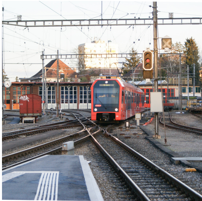
An RBS train from Berne arrives in Solothurn on 15 January 2011. The antenna cable of the ZSL 90 train protection is visible between the rails. Photo: Markus Giger.
