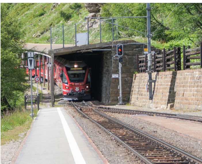
High-risk signals often stand on downhill sections or protect the exit of passing loops. This is Rhaetian Railway's Alp Grüm station on 16 July 2014. Photo: Markus Giger.
