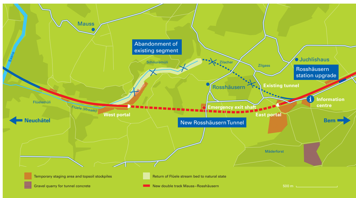
The new Rosshäusern Tunnel passes under semi-rural hills west of Bern. Diagram BLS.
