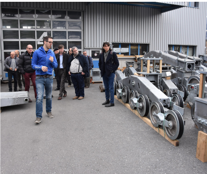
Top left: Daniel Candinas explains the fabrication of large cable wheels in Flums in halves that then go to the destination country, where his company supervises the safety-critical task of welding of the two halves together.
