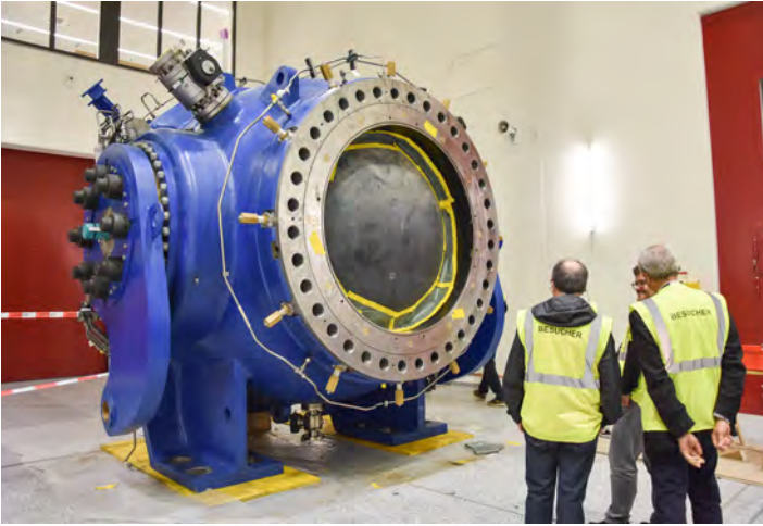
Above left, one of the 180-tonne valves, built for a pressure of 105 bars, whose movable sphere can restrict flow to 30% in 6 seconds and shut completely 36 seconds later.
