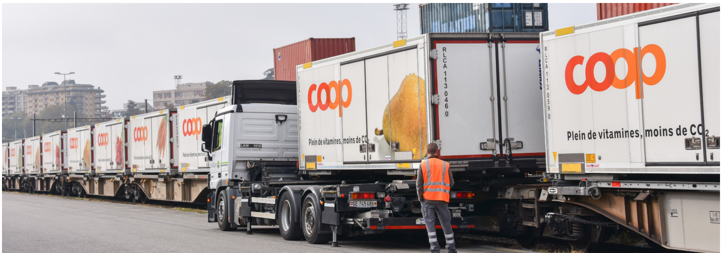
The custom-designed trucks, swap bodies and wagons of the RailCare unit of Swiss supermarket chain Coop enable horizontal loading. Geneva-Carouge, 26 October 2018. Photo George Raymond.
