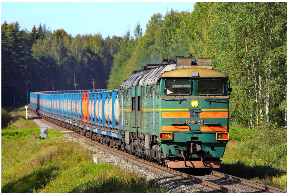
Eastbound tank containers near Ludza, Latvia. The Russian border is 40 km ahead. Both here and in Russia the rails are 1520 mm apart; in China and most EU countries the standard is 1435 mm. Photo © Konstantin Davidoff.
