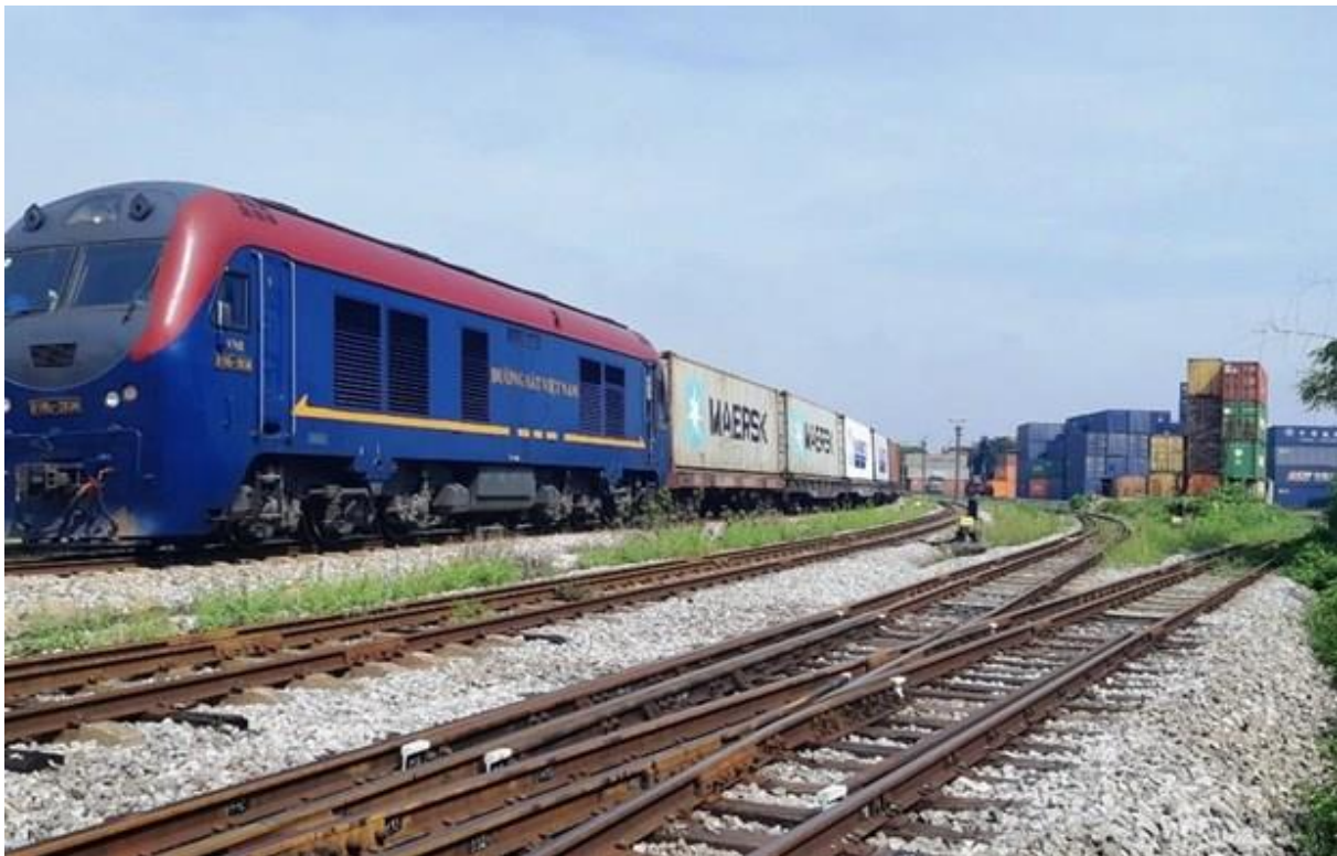
The first container train from Hanoi to Liège, Belgium, leaves Yên Viên station on dual-gauge track (1000 and 1435 mm) on 20 July 2021. Photo VNA reproduced from VietnamPlus, 3 August 2021 .
