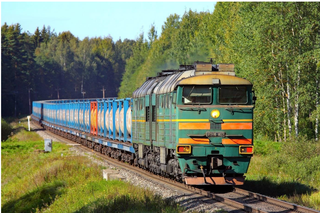
Eastbound tank containers approach Ludza, Latvia, 10 September 2016. The Russian border is 40 km ahead. Here, as in Russia, the rails are 1520 mm apart; in China and most EU countries the standard is 1435 mm. Photo Konstantin Davidov.
