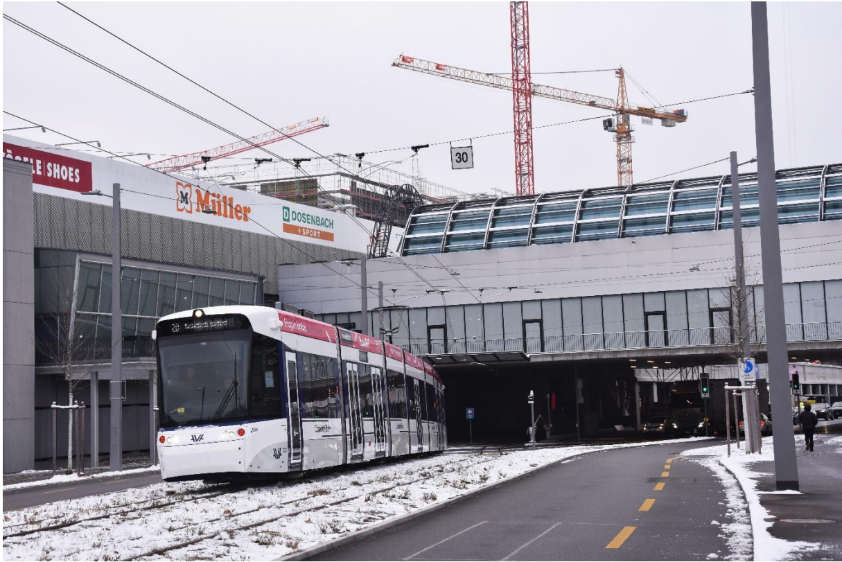
A westbound train accelerates out of the Limmattalbahnhof's station on 12 December 2022 under the Tivoli shopping and development complex in Spreitenbach. Unlike Zurich's trams, which have doors on one side and a single cab and need a loop to reverse, LTB trains are double ended. This saves space at end stations and lets a single set of escalators reach the line's only central platform, here at Shoppi Tivoli station. Photo © George Raymond
