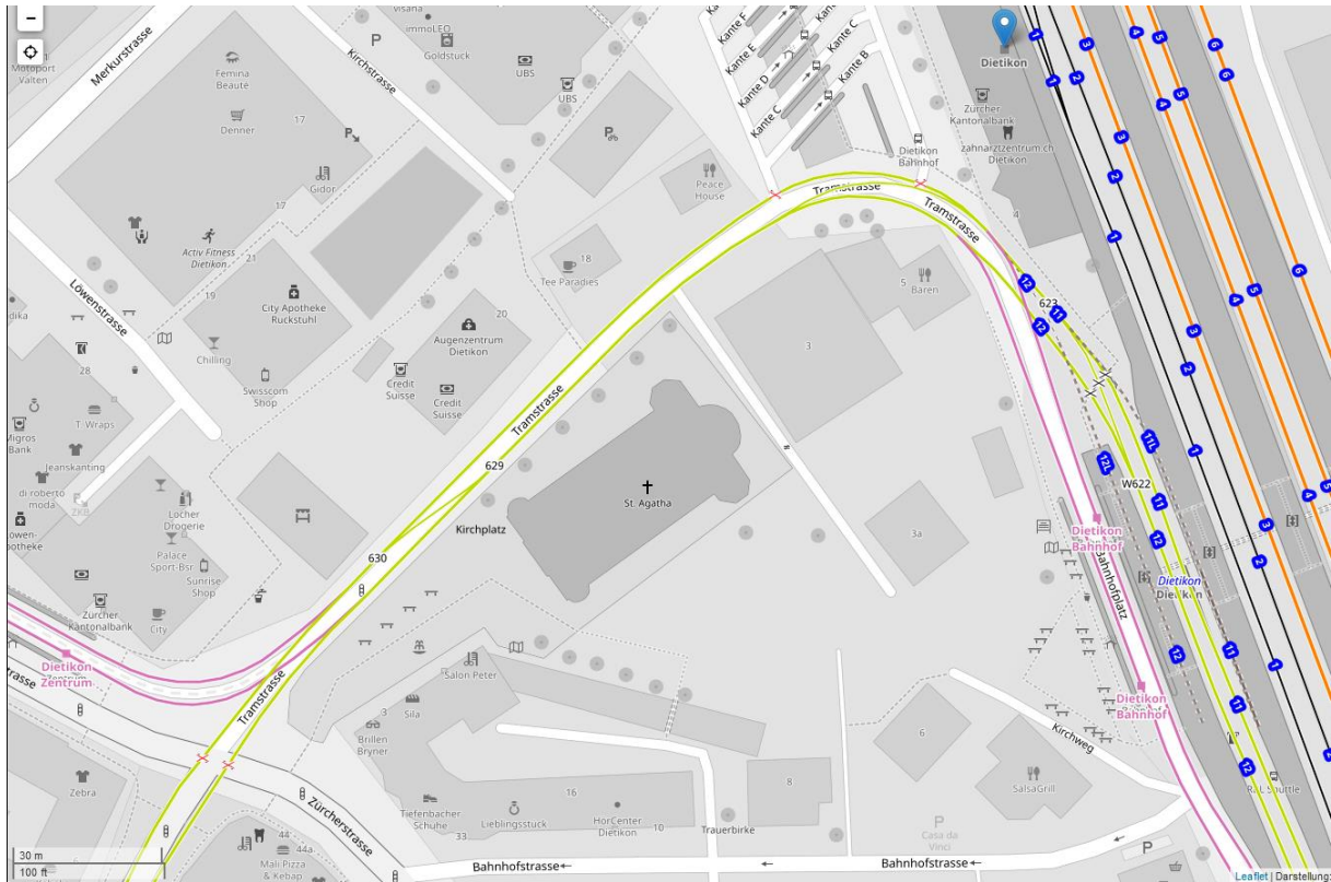
In Dietikon's aptly named Tramstrasse, the shared 160-metre track section of the Limmattalbahn (purple) and the Bremgarten-Dietikon Railway (green). Both connect to S-Bahn and some intercity trains (orange) at SBB's Dietikon station. Source: © Open Railway Map
