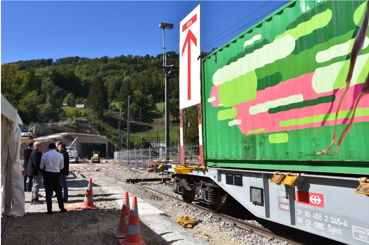
Illustration of clearance for 4-meter semi-trailers riding on pocket wagons on 20 September 2019 at Switzerland's rebuilt Bözberg tunnel, which has since opened. Photo George Raymond.
