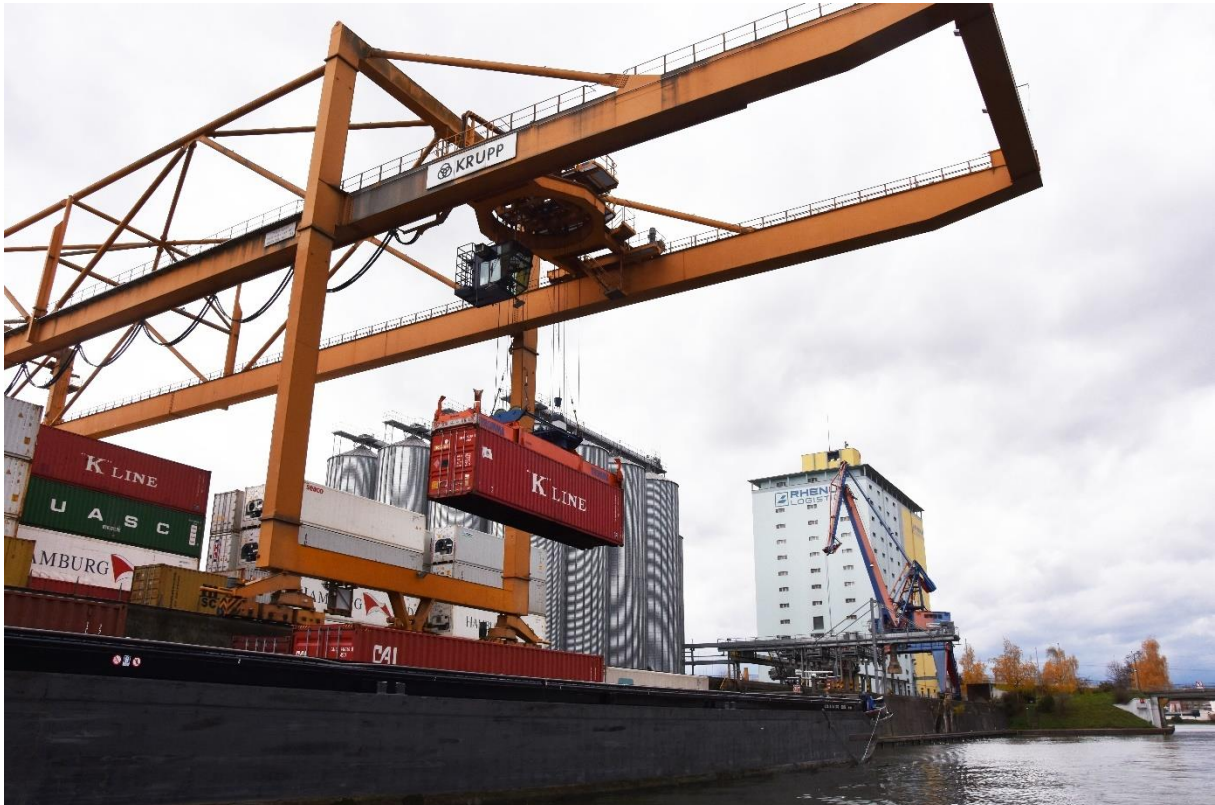
Containers and a Rhine barge in Contargo's terminal on the south side of Basel's Port Basin 2. The crane also serves railway tracks between the water and the container stacks. 18 November 2016. Photo George Raymond.
