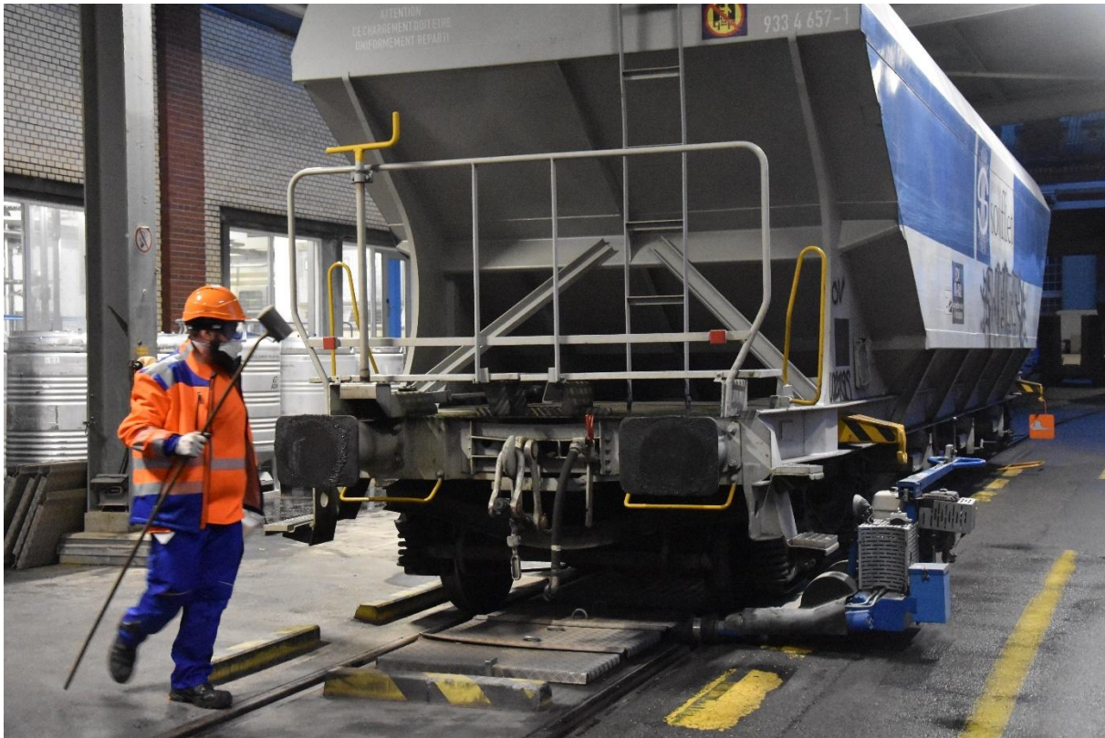
Unloading a wagonload of barley imported from the Dijon area of France at the Feldschlössen brewery in Rheinfelden, Switzerland on 13 November 2023. It is equipped with the standard European standard screw coupler and buffers. Photo © George Raymond.
